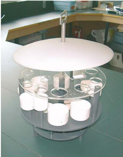
Photo 7. Multiéchantillonneur assemblé. (B.C. Ministry of Water, Land and Air Protection., 2005.)
